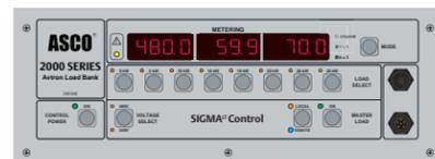
The SIGMA LT "digital" toggle switch local control panel is provided as standard on SIGMA LT load banks. It provides straight forward control along with LED metering and provisions for the optional hand-held control (to enable networking). SIGMA LT only requires a single hand-held to remotely control up to 25 load banks. SIGMA LT load banks of varying load capacities can be networked to provide an extensive range of load.
